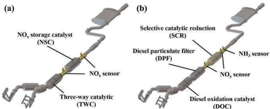
**Fig. 1.5** a Lean combustion technology of gasoline vehicle exhaust purification system; b Diesel vehicle exhaust purification system
