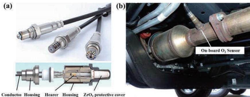
**Fig. 1.4** **a** Structural diagram of on-board oxygen sensor; **b** Working principle of oxygen sensor in automobile exhaust system
