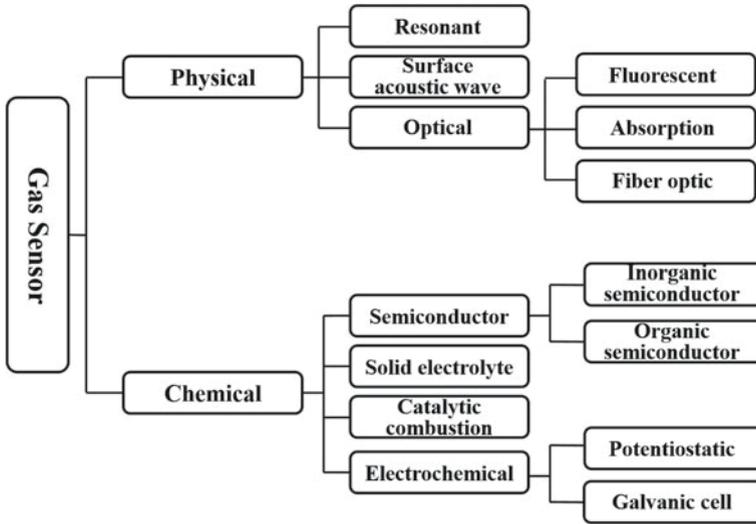
**Fig. 1.3** Classification of gas sensors
